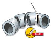
**2** Fit the segments together and glue them to form the curved section required
