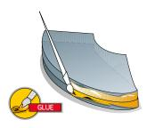
3 Lay one section flat on top of the other and spread MATIBLOCK® glue on the longest edge of both
