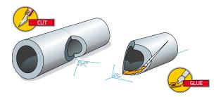
2 Midway along the longest section, make two 45°cuts converging towards the centre of the sleeve. Then make two 45° cuts at one end of the shorter section and apply glue to the cut edges
