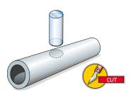
1 Make a hole in the TROCELLEN insulating sleeve using a tube with sharpened rim
