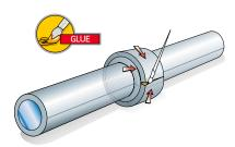
5 The strip which is obtained can then be fitted round the flange, after glue has been carefully applied to the points of contact with the two rings previously fitted
