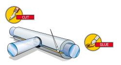
2 Cut the sleeve lengthways and fit it to the pipe. Spread the cut edges with MATIBLOCK® glue and press together
