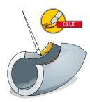
5 Apply glue to the inside edges and allow to dry
