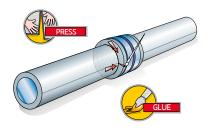
3 After applying MATIBLOCK® where necessary to the insulation and to the flanges, glue the rings of insulation to the side of the flanges
