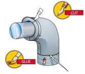
7 Using metal tape as a guide, cut the exposed ends to be at a right angle to the pipe to fit with connecting sleeves
