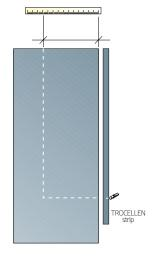
4 Using a strip of **TROCELLEN** of the same thickness, measure the circumference of the two rings of insulation fitted and the distance between them, including the width of the rings themselves. Using these measurements, trace and cut out the rectangular section to cover the top of the flanges
