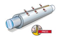
Wait for the glue to dry, then join the two edges, pressing them together to ensure perfect bonding
