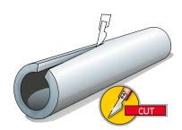
Cut the insulating sleeve lengthways
