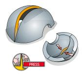
4 When the glue has dried, join the two flat sections, starting by gluing the outside edges and ensuring that the join is perfect on the other side, too
