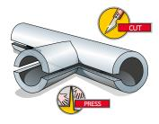
3 Fit the two sections together to make a "T" shaped branch. Cut the sleeve lengthways to allow for fitting
