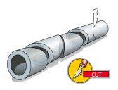
1 Cut a TROCELLEN sleeve into three or four segments with the same angles and rotate each segment cut through 180°
