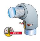
6 Fit the insulating material to the curved section of piping, pressing the internal cut edges together firmly
