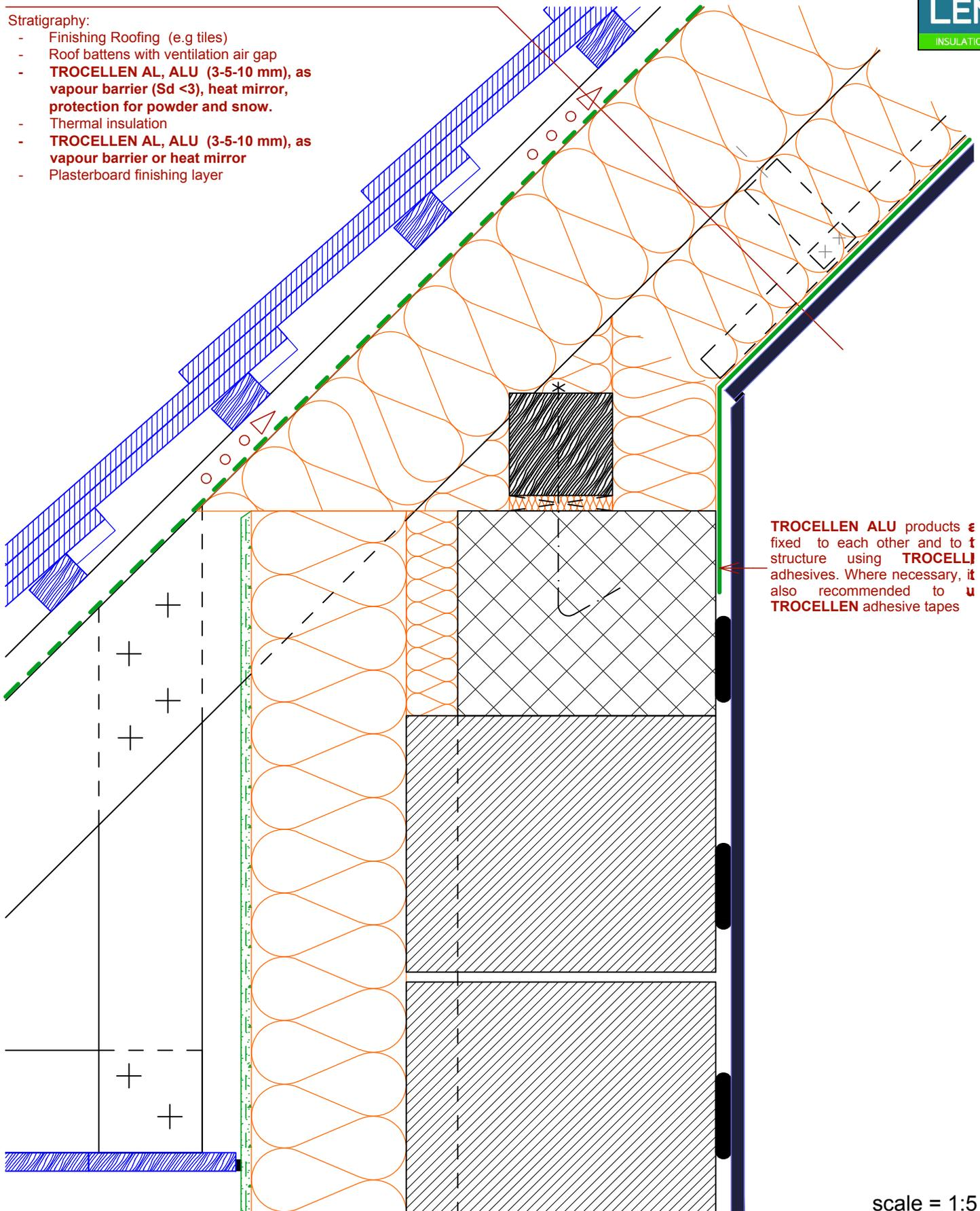
**TROCELLEN ALU** products are fixed to each other and to the structure using **TROCELLI** adhesives. Where necessary, it is also recommended to use **TROCELLEN** adhesive tapes
